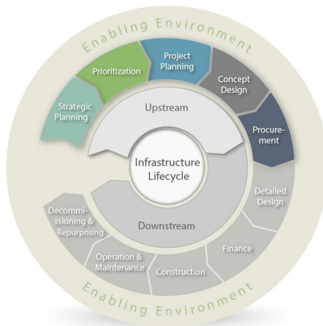
FIGURE 1. THE INFRASTRUCTURE LIFECYCLE FROM NATIONAL, REGIONAL, OR MUNICIPAL STRATEGIC PLANNING AND PRIORITIZATION THAT OCCURS “UPSTREAM” OF ANY SINGLE PROJECT (HIGHLIGHTED IN THIS FIGURE), TO THE DETAILED DESIGN, FINANCE, CONSTRUCTION, AND ULTIMATELY DECOMMISSIONING OF INDIVIDUAL PROJECTS “DOWNSTREAM”. 3
